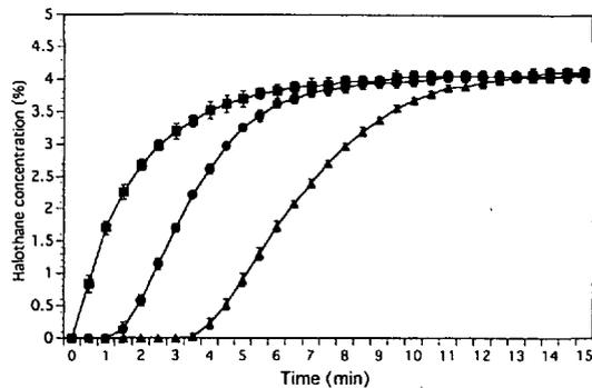
**Fig 1** Rate of increase in halothane concentration in anaesthetic chamber (chamber size=  $45.5 \times 30.5 \times 30.5$  cm). Fresh gas flow rate, 5 l/min, 4.3% delivered halothane concentration, sampling catheters placed at (a) 5 cm (■), (b) 15 cm (●) and (c) 25 cm (▲) above the base of the chamber
