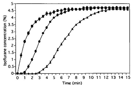
**Fig 2** Rate of increase in isoflurane concentration in anaesthetic chamber (chamber size=  $45.5 \times 30.5 \times 30.5$  cm). Fresh flow rate, 5 l/min, 4.7% delivered isoflurane concentration, sampling catheters placed at (a) 5 cm (■), (b) 15 cm (●) and (c) 25 cm (▲) above the base of the chamber
